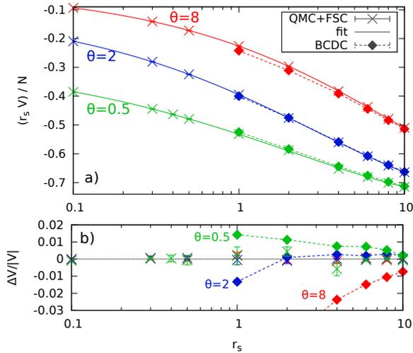
Figure S5: Potential energy of the warm dense electron gas in the TDL. Panel **a**) shows our new corrected data for three temperatures, the fits to our data (see Eq. (S.3)), and the data by Brown *et al.* (BCDC), taken directly from their supplement. Panel **b**) shows the corresponding relative deviations to the fits to our data.
