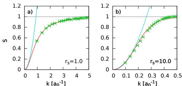
Figure S1: Static structure factors of  $N = 66$  electrons at  $\theta = 2$  for a)  $r_s = 1.0$  and b)  $r_s = 10.0$ : QMC data (green crosses), STLS (red) and  $k \rightarrow 0$  expansion of the the RPA SF (light blue).
